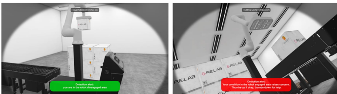
Figure 79 AR Operator Recognition App. Feedback through an augmented interface in collaborative scenarios. The AR application displays personalized recognition messages and safety alerts directly through the operator's smart glasses.
