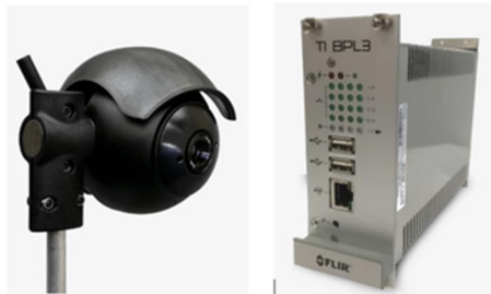
Figure 49 FLIR/CiT One RSU – compact V2I communication unit with integrated antennas
