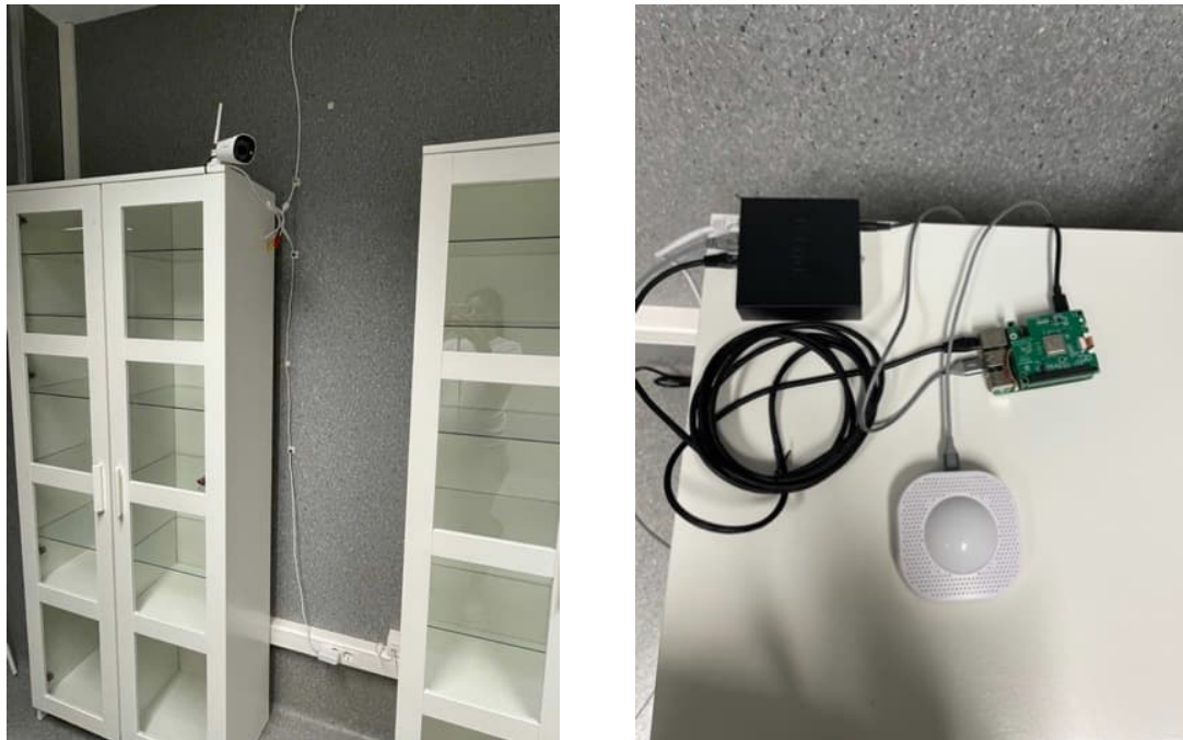
Figure 3 RGB camera (left) and edge processing element (right) for bradykinesia monitoring at IRBLL
