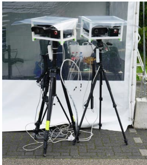
Figure 54 Imec sensor boxes with visible and thermal camera, radar and lidar
