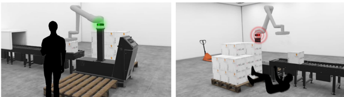
Figure 78 Operator Mirroring Ring. Examples of interaction with the robot in ordinary and anomalous scenarios. The LED-based interface provides immediate visual feedback on operator recognition and the state of collaboration.
