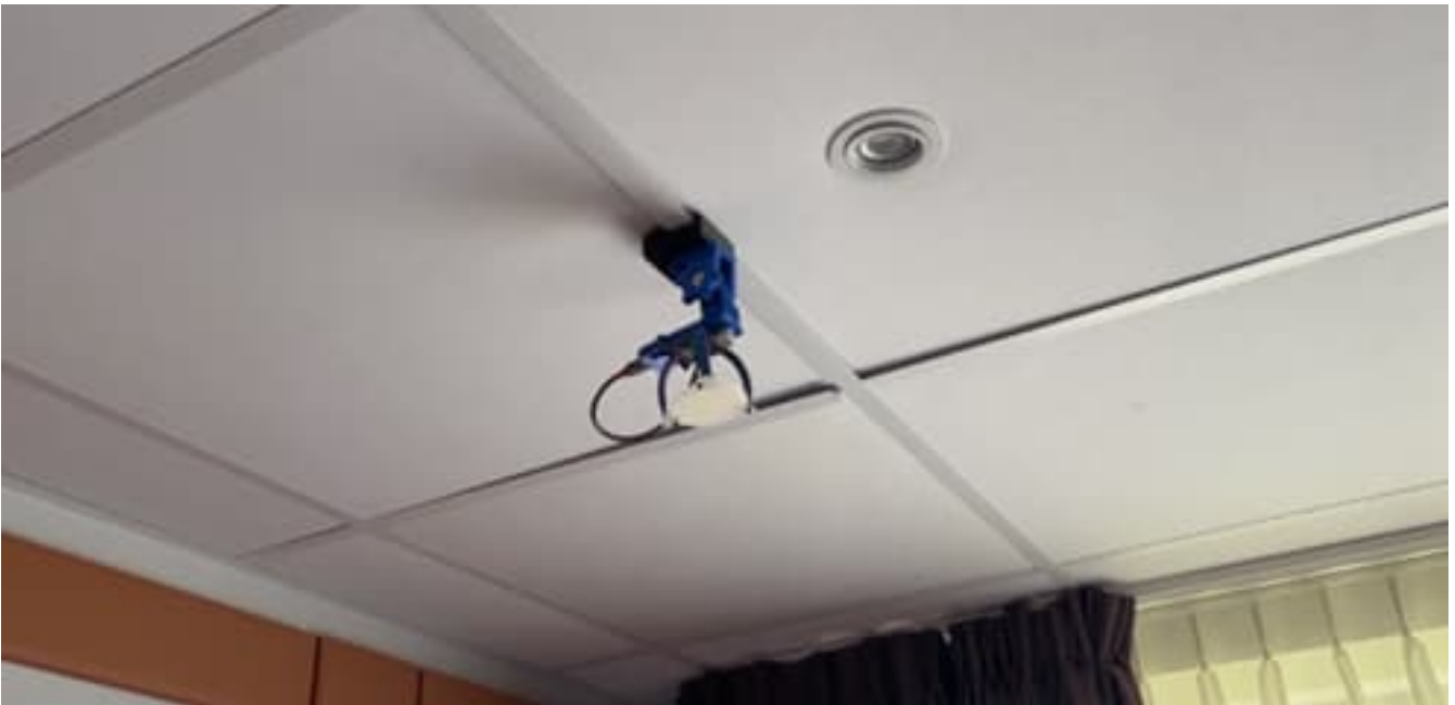
Figure 19 When the ceiling plates are in place, the VTT radar is hidden above, and the Infineon radar is as shown in the picture.
